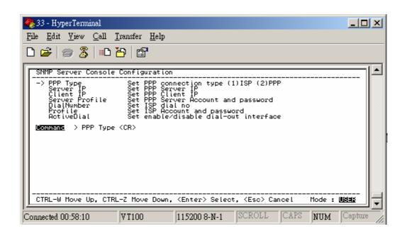
16. Arrow down to PPP Config and hit enter. Enter in the ISP dial number, the ISP account/password and the enable/disable dial-out interface (not required). Hit the "Escape" key to return to the main menu.
